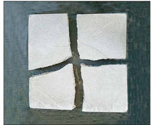
Unreinforced concrete slab after a single impact drop test of 12,000 pound force.
